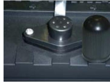
The winch now has an integrated cut off switch, either the wireless activator or the lead remote must be installed for the winch to work.
